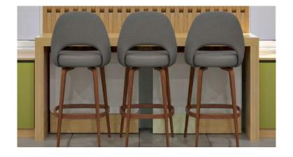
Bar counter made out of 20mm thk ply boxing finished with laminate - 1880mm x 500mm x 900mm - 75mm thickness
